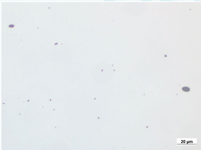
Low Alloy Steel 42CrMo4+QT, 330 HV, BF, 500x
